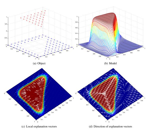
Figure 1: Explaining simple object classification with Gaussian Processes
