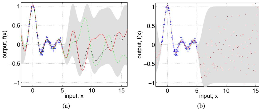
Figure 2: Learning the  $\text{sinc}(x)$  function from 100 noisy observations (plusses) using 40 basis functions with shaded area showing 95% (noise free) posterior confidence area. In panel (a) the SSGP method with three functions drawn from the posterior is shown. In (b) the same data for the FITC method with samples (dots) drawn from the joint posterior.
