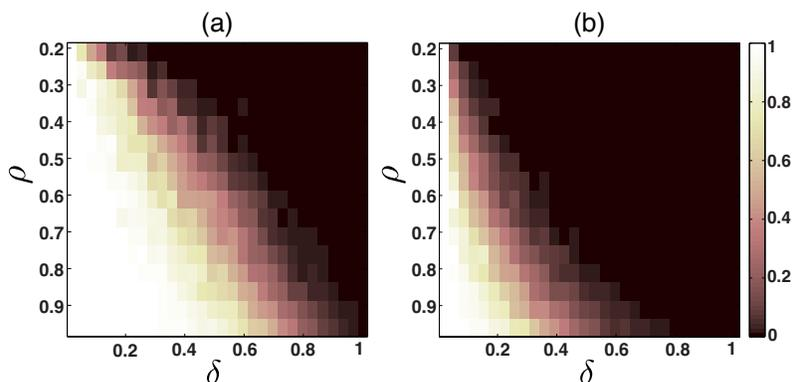
Figure 7: Phase transitions for OMP and NN. The probability of EFS for orthoblock sparse signals for OMP (a) and NN (b) feature sets as a function of the oversampling ratio  $\rho = k/d$  and the overlap ratio  $\delta = q/k$ , where  $k = 20$ .
