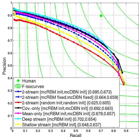
Figure XXII: Deeper Network Prediction Performance Dissection on the **BSDS500 (Grey-Scale)** as Measured by Precision-Recall Curves. The legend numbers denote the maximums of the curves w.r.t. the ODS F-measure (left), and the average precision (right).
