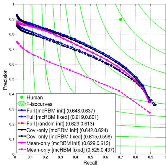
Figure XXI: Shallow Network Prediction Performance Dissection on the **BSDS500 (Grey-Scale)** as Measured by Precision-Recall Curves. The legend numbers denote the maximums of the curves w.r.t. the ODS F-measure (left), and the average precision (right).
