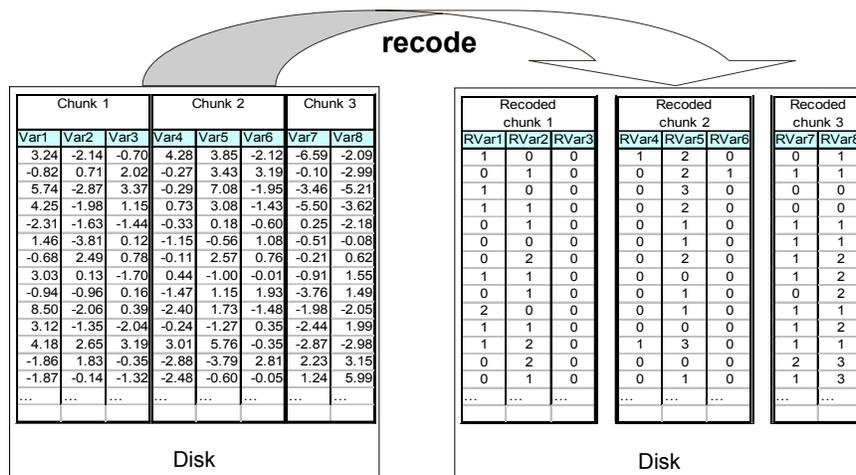
Figure 2: Recoding: the input file on disk is read and recoded once, and several recoded chunks of variables are written on disk.
