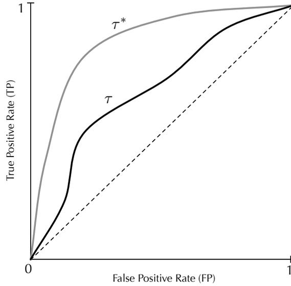
Figure 3: Example of an ROC diagram showing an ROC curve for an arbitrary statistical test  $\tau$  (middle, bold curve) as well as an optimal statistical test  $\tau^*$  (top, grey curve). The dashed line represents the ROC curve for a random, or uninformative statistical test.
