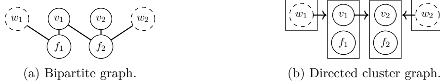
Figure 3: The bipartite graph in Figure 3a is associated with the constraints in Example 4. Exogenous variables are indicated by dashed circles. The directed cluster graph that is obtained by applying Algorithm 1 is shown in Figure 3b.
